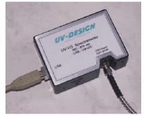
The USB Miniature Fiber Optic Spectrometer, is a revolutionary small plug-and-play spectrometer and features these key innovations:
