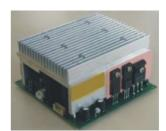
The EVG UV 12-25 AC is a fully electronic, adjustable AC ballast unit for UV-lamps from approx.  $0.4 \, \text{kW} - 1.2 \, \text{kW}$  nominal power and specially designed for industrial use. It is specially tuned to operate with mercury discharge UV-lamps of  $5-25 \, \text{cm} \, (2"-10")$  arc length. Dark phases during the zero axis known from standard, sinus shaped power supplies are eliminated by operating the lamps with a square-wave current.
