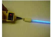
The Lamp Tester LT 200 is a compact, versatile test instrument for swift checking of all gasfilled low pressure and high pressure dischagre lamps
