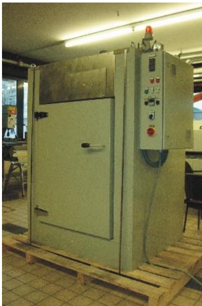
Forced Convection Box Oven 640 L Temperature range 70 – 300°C
