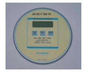
The UV-3C-T Integrator 120-10 is a self-contained, high quality UV measuring instrument. It is designed to measure and display peak UV intensity, UV dosage and temperature in the UV curing process. Thank to its special dimensions it is particularly suitable for the CD and DVD production.
