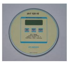
The UV-T Integrator 120-10 is a self-contained, high quality UV measuring instrument. It is designed to measure and display peak UV intensity, UV dosage and temperature in the UV curing process. Thank to its special dimensions it is particularly suitable for the CD and DVD production
