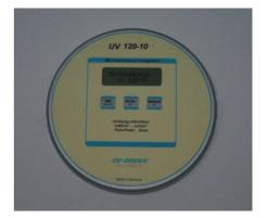
The UV Integrator 120-10 is a self-contained, high quality UV measuring instrument. It is designed to measure and display peak UV intensity and UV dosage in the UV curing process. Thank to its special dimensions it is particularly suitable for the CD and DVD production
