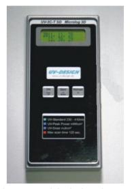
The UV-2C-T Power Integrator is a small, self-contained, high quality UV measuring instrument. It is designed to measure, record and display peak UV intensity (mW/cm²), UV dosage (mJ/cm²) and temperature in the UV curing process.
