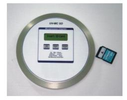
The UV-MC SD Microprocessor Integrator is a self-contained, high quality UV measuring instrument. It is designed to measure, record and display peak UV intensity and UV dosage in the UV curing process.
